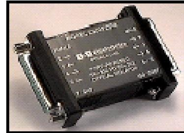
The Model 232SPOP4 optically isolates four RS-232 lines. The isolator has a DB25S female connector on the DTE side and a DB25P male connector on the DCE side of the isolator. Signals pass through the isolator as follows:
